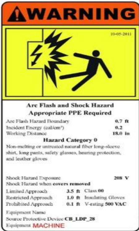
Arc flash hazard warning label
