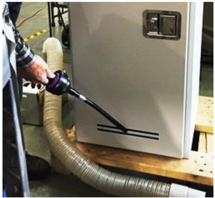
Gas cab tracer gas test
