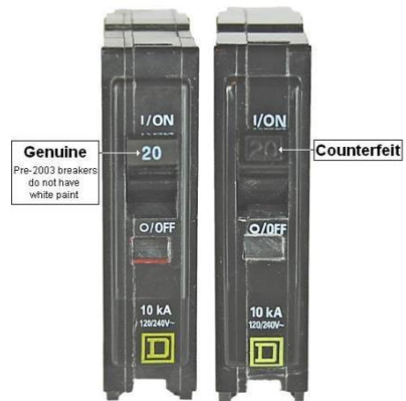
Counterfeit circuit breaker on the right
