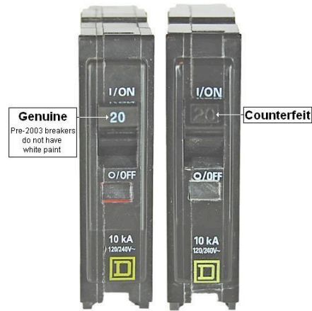
Counterfeit circuit breaker on the right
