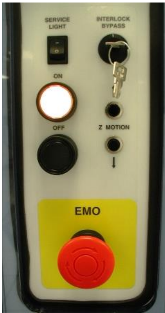
Red EMO on yellow with interlock bypass key
