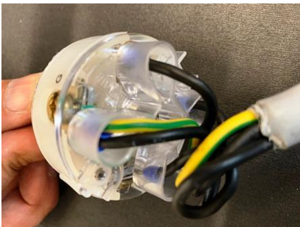
Neutral and ground connected
