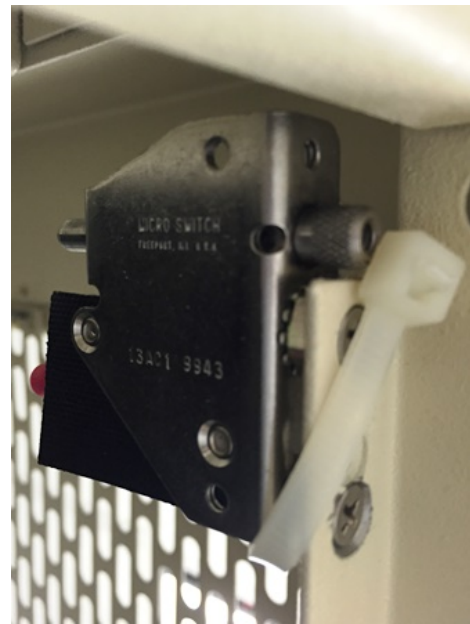
Door interlock should not be easily defeated
