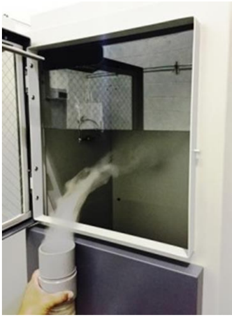
Gas cab ventilation sweep test
