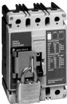
Circuit breaker with hasp – courtesy of Eaton. NEC 110.25 states that the provisions for locking shall remain in place with or without the lock installed.
